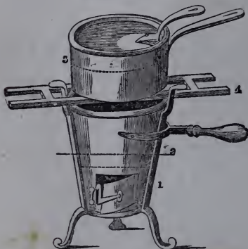
Portable French Furnace, with Stewpan and Trevet.
